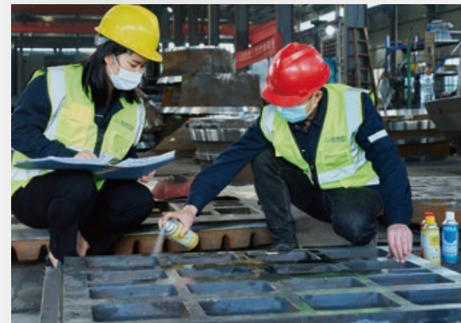
着色探伤 Dye Penetration Inspection
